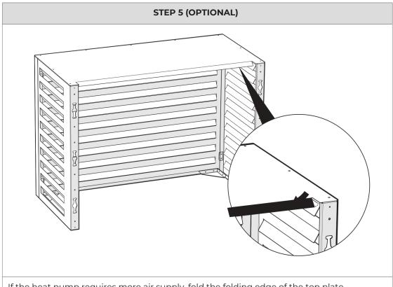
If the heat pump requires more air supply, fold the folding edge of the top plate downwards.
