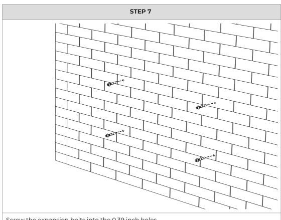
Screw the expansion bolts into the 0.39 inch holes.
