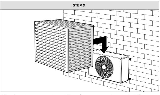
Place the enclosure over the air conditioning/heat pump onto the expansion bolts.
