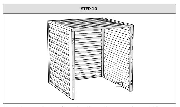
Screw the cover to the floor using the 8 mm holes at the bottom of the cover. Make sure to use a connection appropriate for the floor surface.
