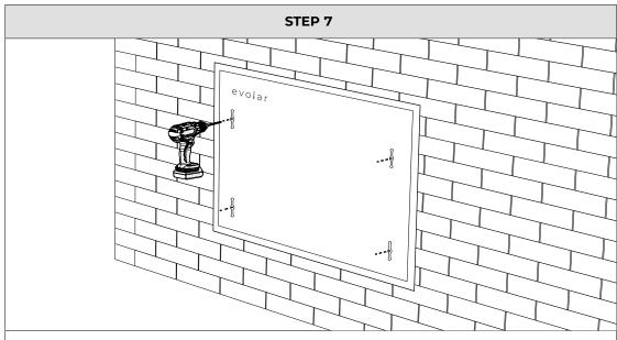
Drill 10 mm (0.39 inch) holes in the wall around your air conditioning/heat pump using the drilling template.
