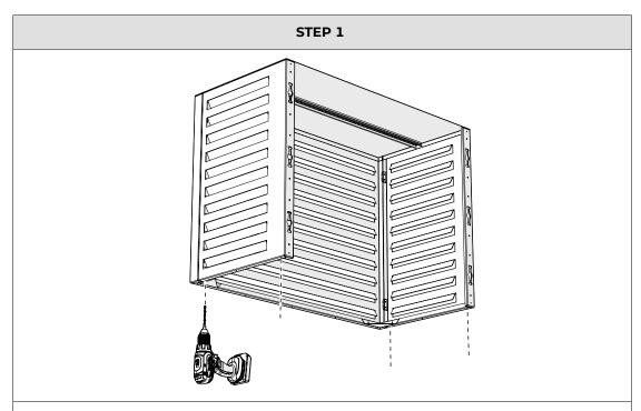
Some Evolar covers already have pre-drilled holes. If not, drill 8 mm (0.31 inch) holes at the corners underneath the enclosure.
